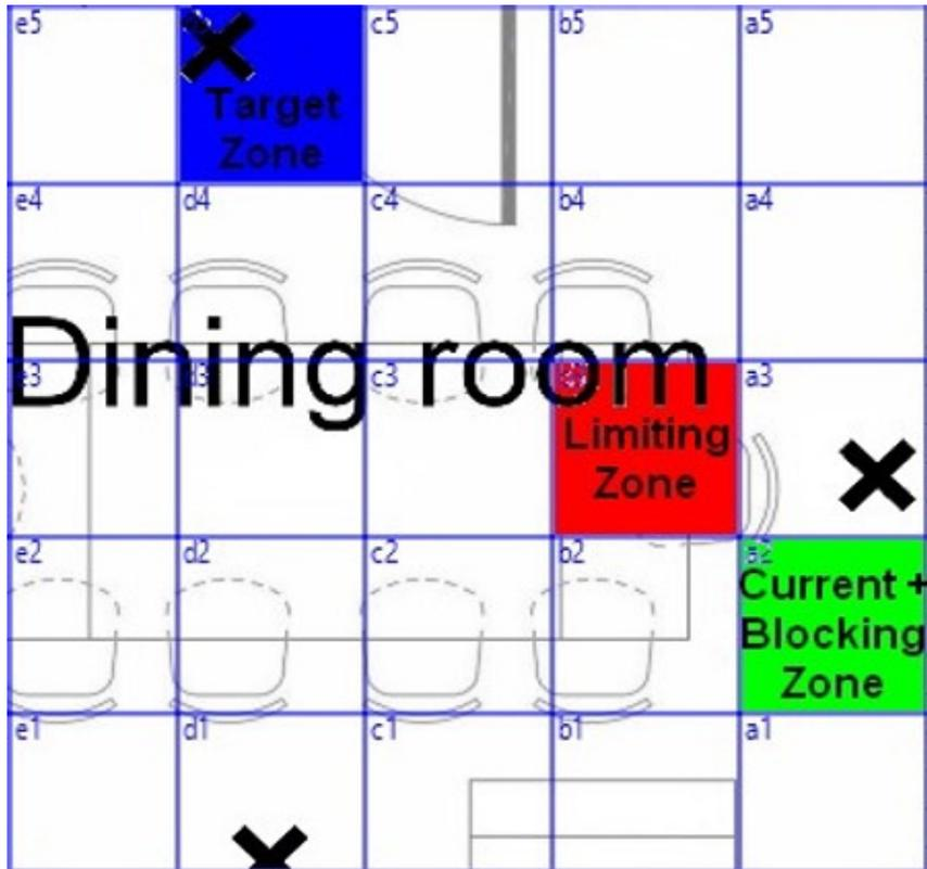
In green is the current zone and the one predicted by the blocking filter. In red is the zone predicted by the limiting filter while in blue is the zone predicted by the random forest.
